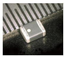
MCP2016D series  $(2.0 \times 1.6 \times 1.0 \text{mm max})$
